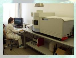
The measurements were performed with inductively coupled plasma-optical emission spectrometer (ICP-OES) Dual View Optima 2000, Perkin Elmer, USA
