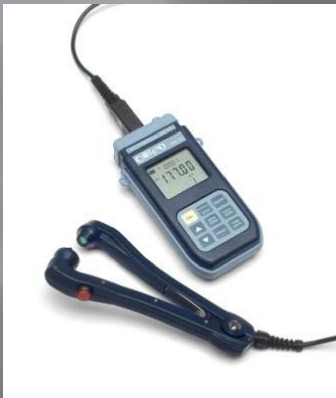
Polyphenolic Meter Alcyone PM-03 ( Caeleno, Italy )
